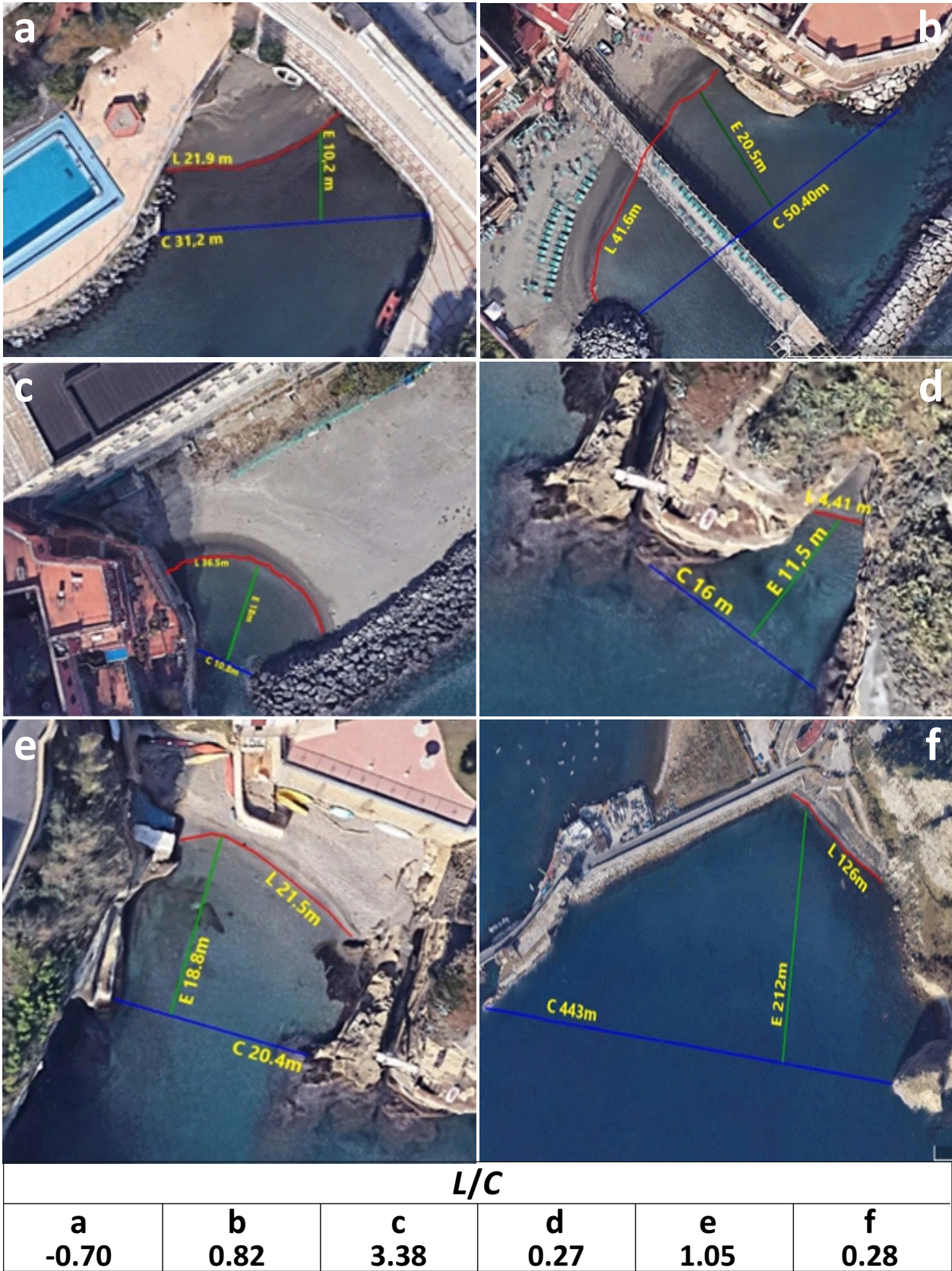
Figure 7: Morphometric parameters of the six urban beaches (after Google Earth Pro 2023): a, Circolo Relax, b, Bagno Sirena, c, Spiaggia delle Monache, d, Spiaggia delle Telline, e, Cala della Zafferana, f, Coroglio. L, length, C, mouth of the bay, E, embayment, and L/C ratio for the shore line shape.
