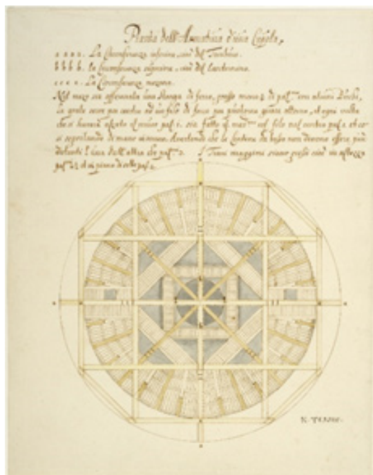
102 Fig. 9: Nicodemus Tessin il giovane, Scaffolding for a Dome with explanatory text in Italian, Scaffolding in the Dome of St. Peter's Church, Rome , Stoccolma, National Museum, NMH CC 749, NMH CC 2253 recto.
