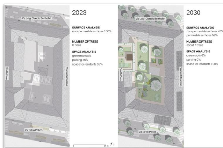
Fig.22 Before and after, project inner courtyard
