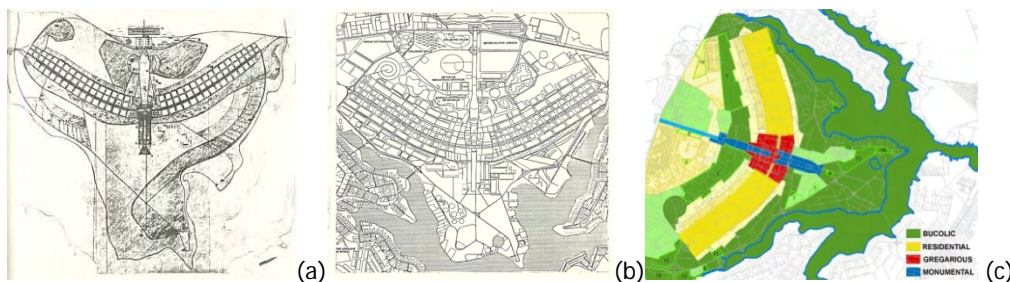
Figure 1 - Original Pilot Plan, submitted in the competition (a), and Pilot-Plan built (b). (Source: Lúcio Costa, Brasília 57-85, 1985). Scales bucolic (green), gregary (red), residential (yellow) and monumental (blue), (Adapted from SEDHAB, 2013)
