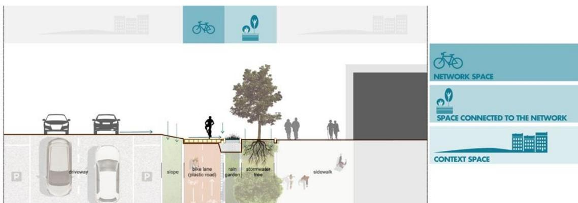
**Fig.4 Zwolle, section of the Plastic Cycle Road in Deventerstraatweg**
