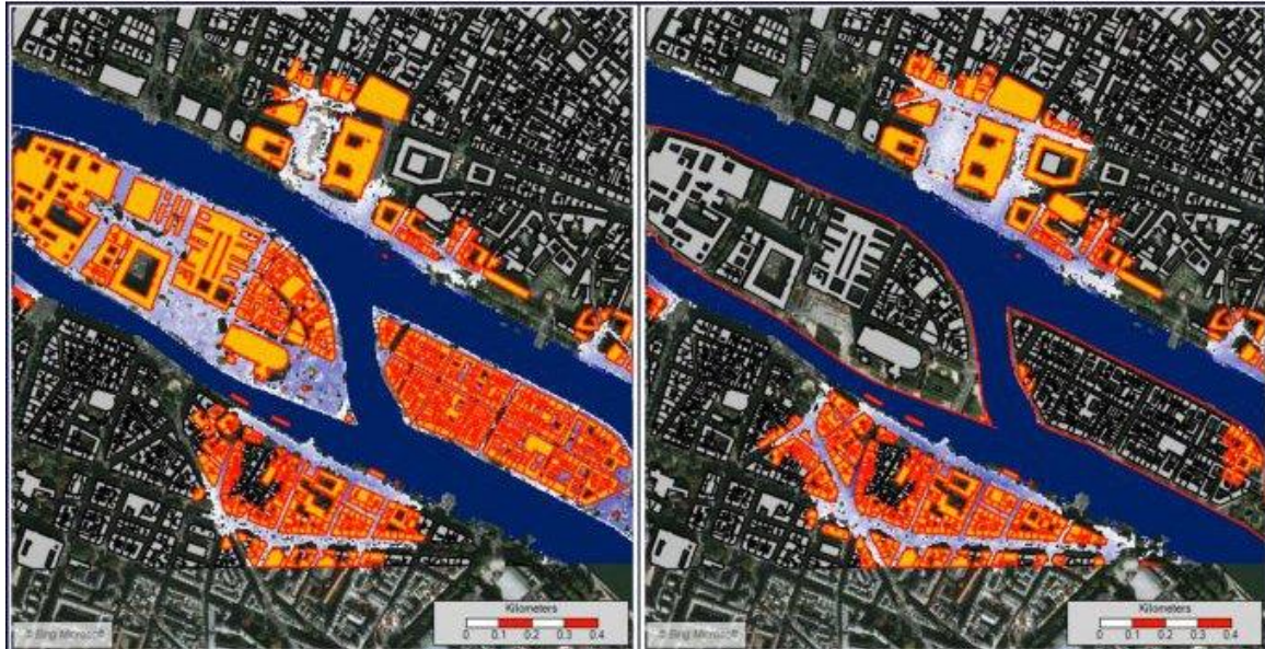
Fig.4 The Digital Twin of Lisbon. Flood simulation in downtown: two different scenarios
