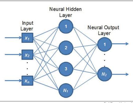
Fig.1 The architecture of 3 layer MLP Network
