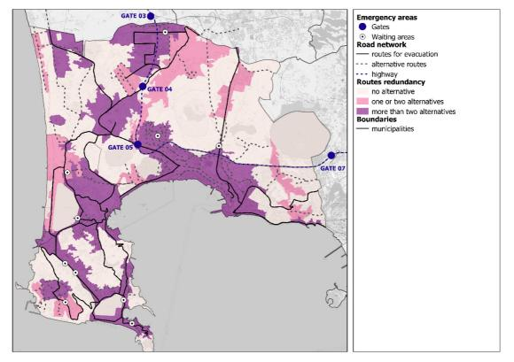
Fig.10 Redundancy of the road network
