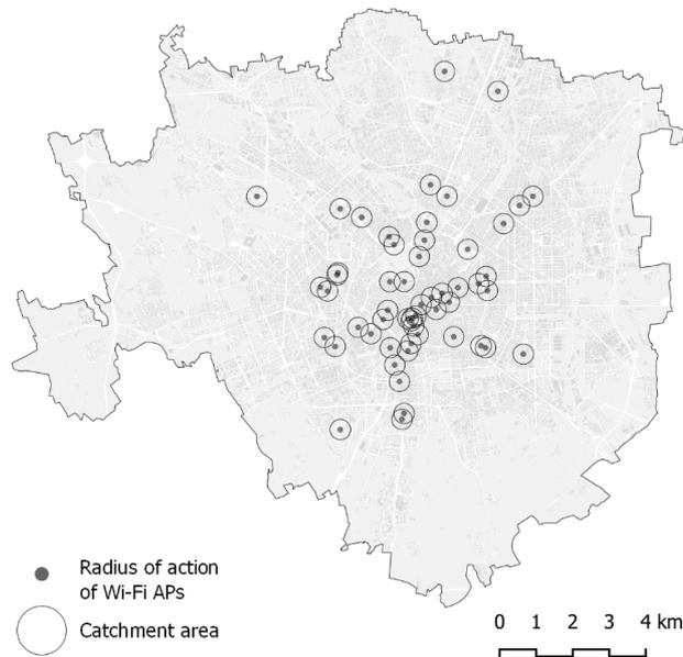
**Fig.1 The location of the 55 Wi-Fi APs, with related radius of action ( $r = 80\text{ m}$ ) and catchment areas ( $r = 280\text{ m}$ )**
