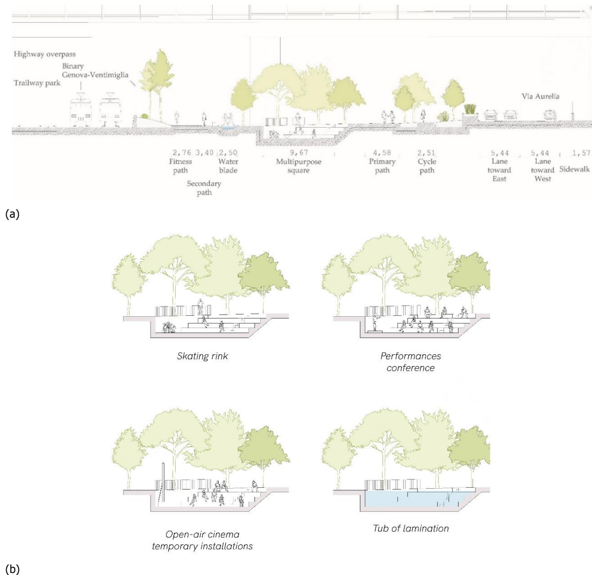
Fig.11 (a) Cross section of the project and (b) The functions of the multi-purpose square
