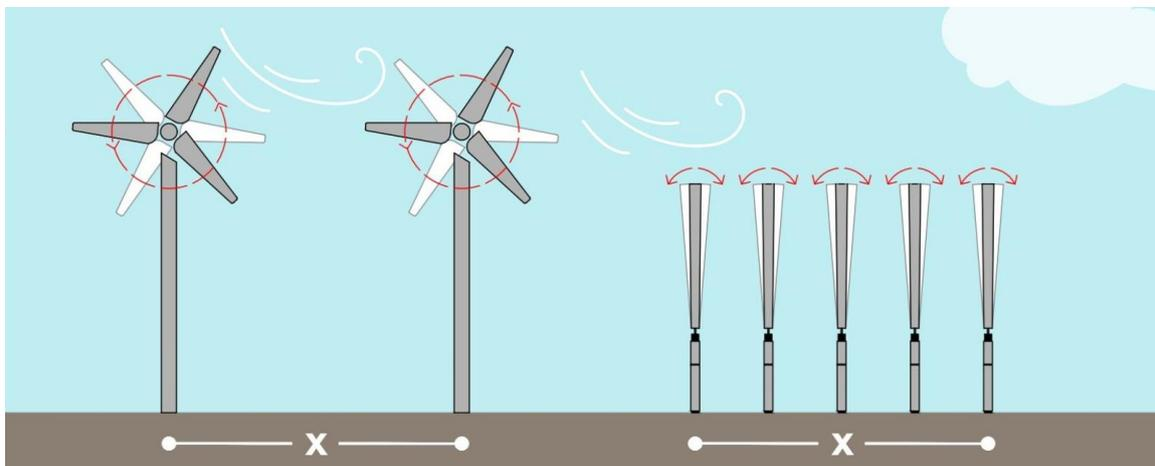
**Fig.5 Comparison of technology on wind turbines and Vortex devices**
