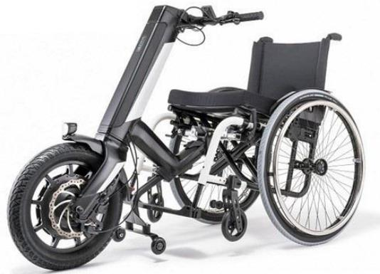
**Fig.8 Manual wheelchair electrified by a front power assist drive unit with steering column: medical assistive device or motor vehicle? (source: Officine Ortopediche S.r.l.)**
