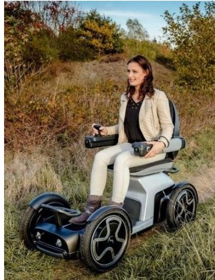
**Fig.7 This device should be classified as mobility scooter because of the presence of a steerable front axle, even if it steers with a joystick (source: scoozy.nl; photographer: Jorrit Lousberg)**
