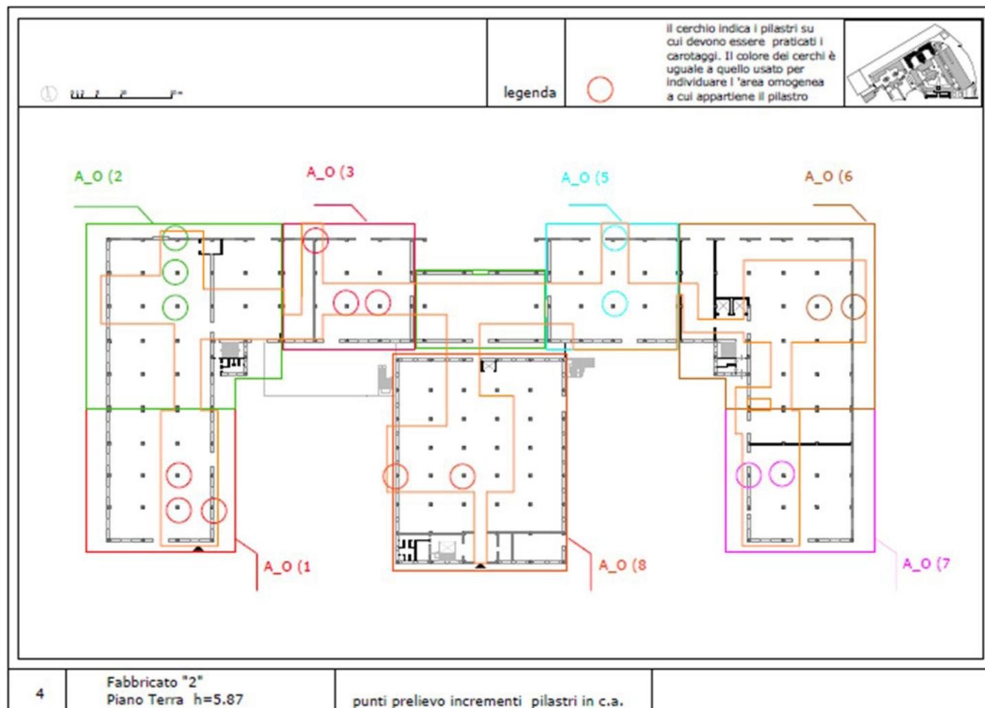
Fig. 4 - Building n.11: homogeneous Areas and sampling point.
