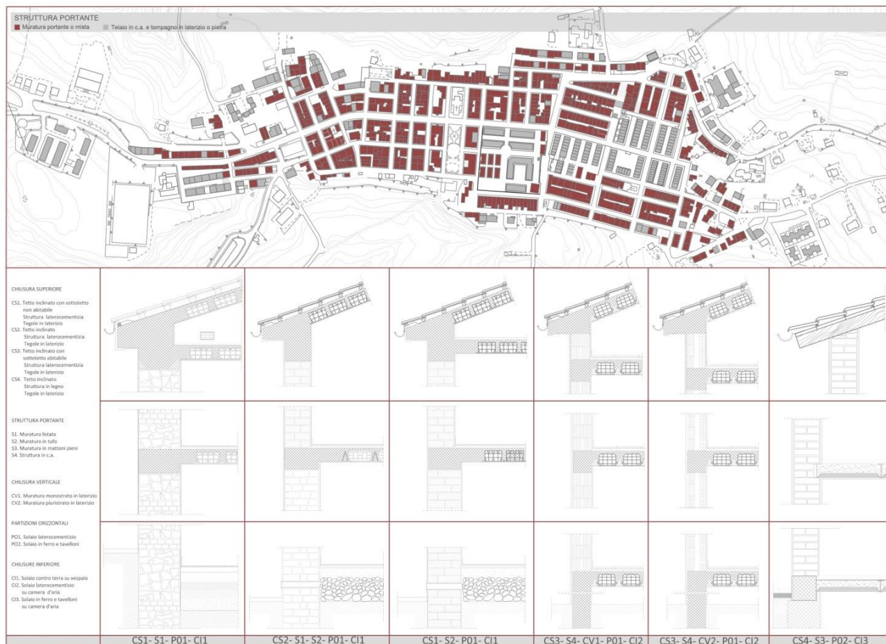
Figure 3: Residential building. Structural typologies analysis
