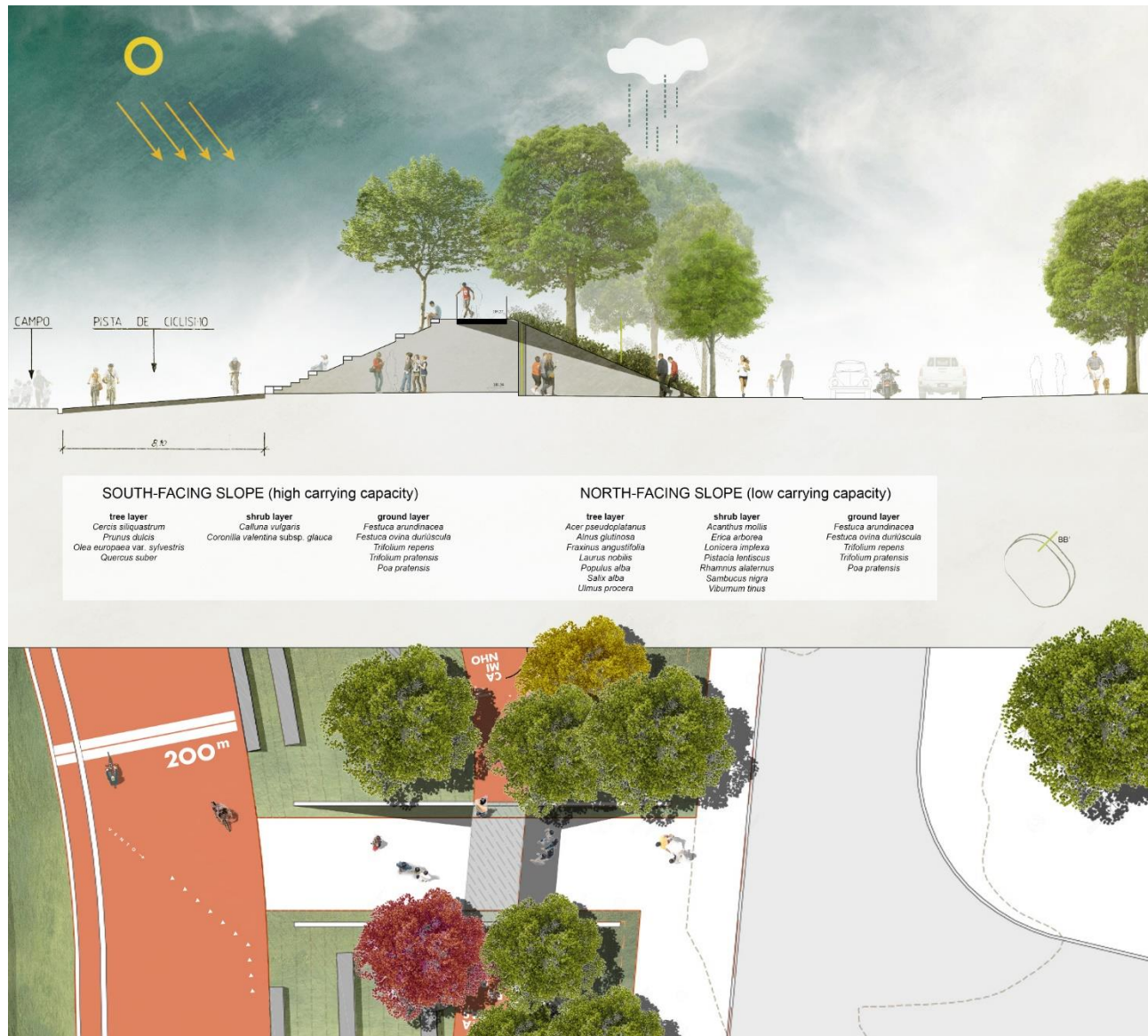
Figure 6: Proposed terrain profile and existing wall (---) rehabilitated for land support. Source: Copyright 2017 Eduardo Costa Pinto, Frederico Vital Soares
