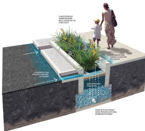
Figure 1: Three-dimensional view of a Stormwater Planter. Source: City of Philadelphia Green Streets Design Manual, 2014
