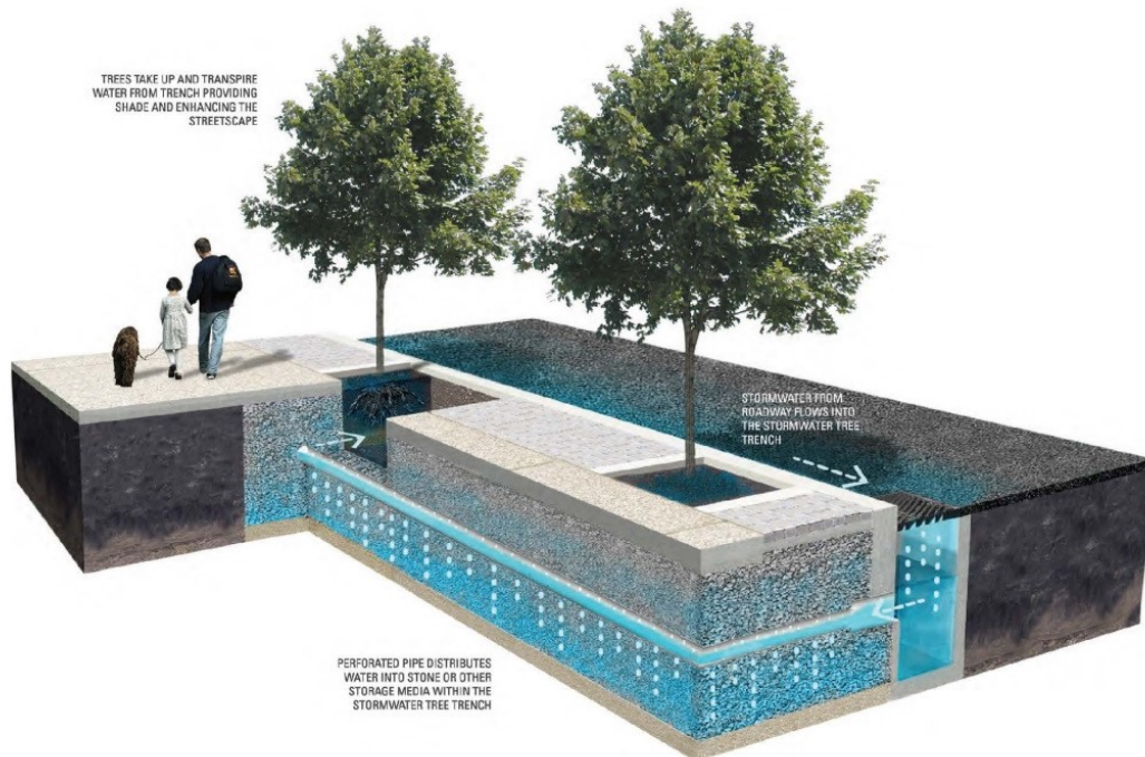
Figure 4: Three-dimensional view of a Stormwater Tree Trench. Source: City of Philadelphia Green Streets Design Manual, 2014
