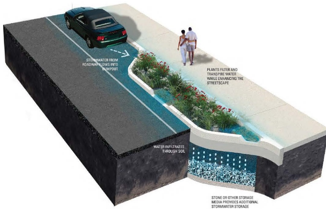
Figure 2: Three-dimensional view of a Stormwater bump-out. Source: City of Philadelphia Green Streets Design Manual, 2014
