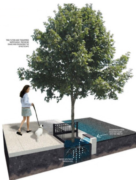
Figure 3: Three-dimensional view of a Stormwater Tree. Source: City of Philadelphia Green Streets Design Manual, 2014
