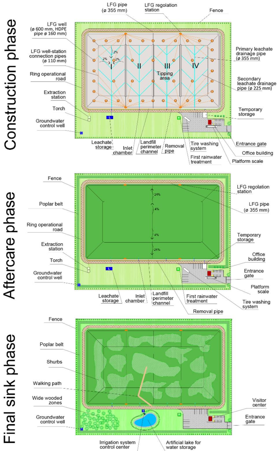
**Figure 3:** Scheme of a landfill area during (a) the operation phase, (b) the aftercare phase and (c) the final sink phase where it is requalified as a natural area. *Source: Authors' elaboration.*
