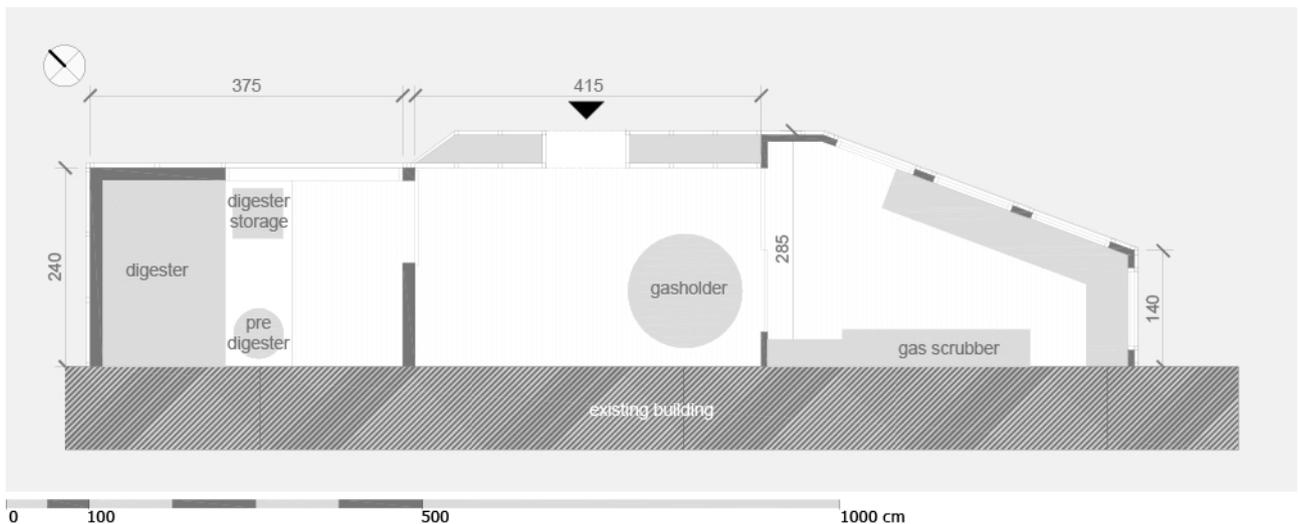
**Figure 6:** Camley Street Park, London (UK). The preliminary project of the micro-AD shows the dimension of the technological components and the equipment designed. Source: acknowledgment to Rokiah Yaman, Director of Community by Design, London, UK, for the material provided.
