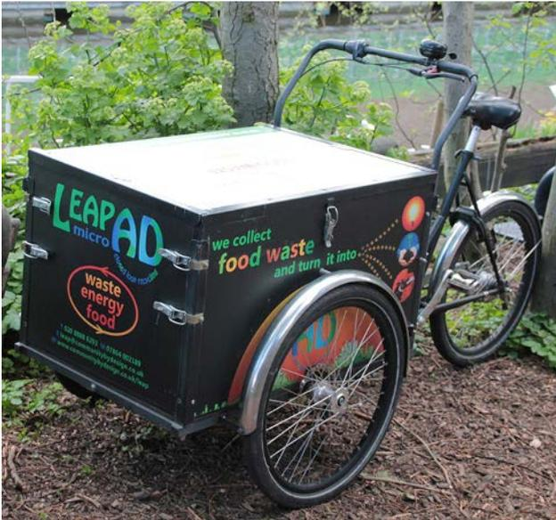
**Figure 7:** Camley Street Park, London (UK). Cargo bike is used for food waste collection direct to Camley Street Park anaerobic digester. The cargo collects 100 kg of food waste has a speed of 15/20 km/h and is used in an area of 3,2 km of radius. *Source: photo by Pracucci, 2017.*
