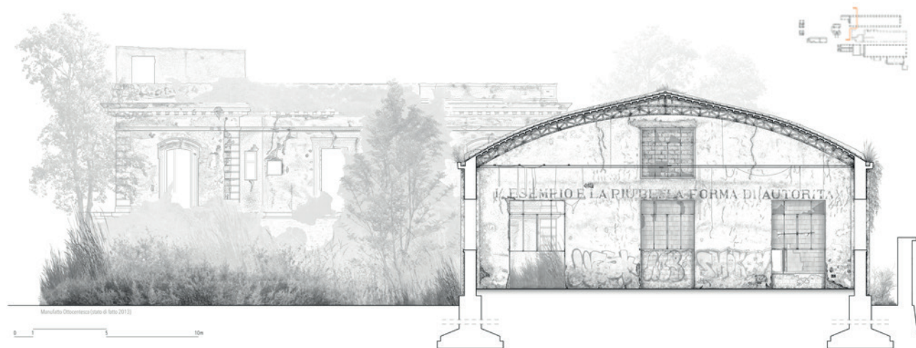
Figure 10: Preservation survey of the first Kerasav's warehouse: south counter-façade. Source: own elaboration.
